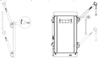
Step: Pull up the 7-shaped knob (59) to unlock, slide the arm up and down to required height; Then release the 7-shaped knob (59) to lock the position. There are 11 heights to choose from (A-K)
