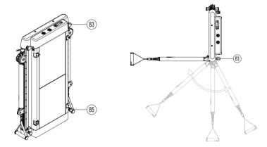
Step: Loose plum knob (83) firstly, keep puling the aluminum pull-pin (85) to unlock, rotate the arm horizontally to the required position; Then release the pull pin (85) to lock the position, and fasten the plum knob (83). There are 5 angles to choose from (-90°,0°,30°,60°,90°)
