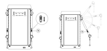
Step: Slide the adjuster (74) to unlock by following the arrow direction, the arm rotates on the vertical plane, and adjust it to the proper position; Then release the adjuster (74) to lock the position; There are 9 levels to choose from (1-9). NOTE: In case you find it difficult to slide the adjustment key, lift the arm a little bit for easy operation.
